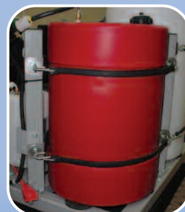
12 US Gallon ( 47 l) Gasoline Tank
