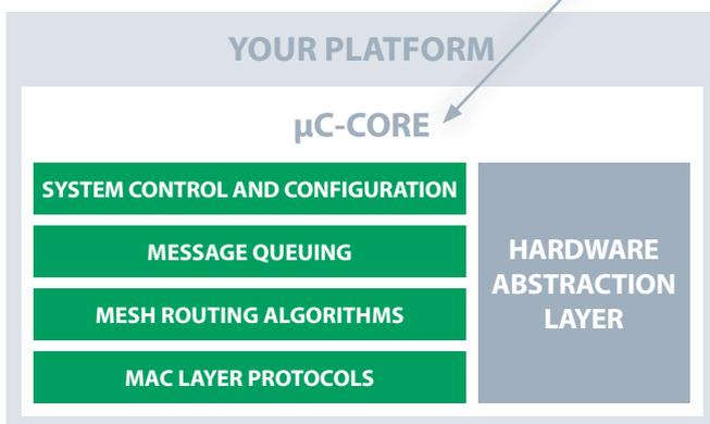
The software framework developed by CRL has a unique modular design making it possible to easily adapt the mesh implementation to varied platforms, ad hoc routing algorithms and services. The algorithms that handle the ad hoc routing/ Mesh protocol) in the mesh are all encapsulated in modules with sophisticated and dynamic interfaces that can be exchanged as plug-ins to the framework.
