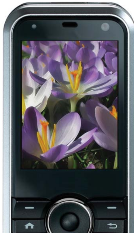
Polysilicon AMOLED with IGNIS AdMo-p™ technology (mura-free)
