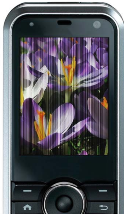
Polysilicon AMOLEDs with no compensation (severe mura)
