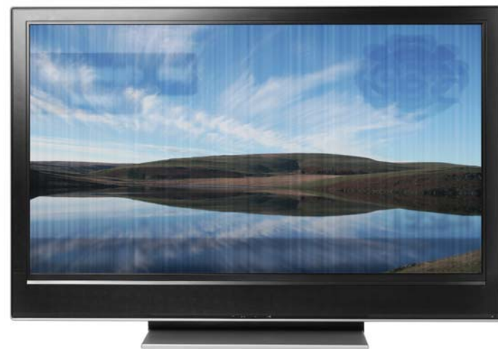
Conventional polysilicon AMOLED televisions show mura and burned-in text and graphics
