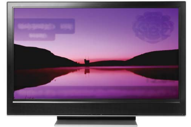
Conventional amorphous silicon AMOLED televisions show burned-in text and graphics
