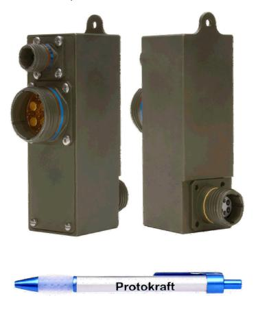
Designed to operate in harsh environments, these media converters feature excellent thermal characteristics, high tolerance to vibration and shock and corrosion resistant aluminum housings for exceptional EMI/RFI performance. Standard case operating temperature range is -40°C to +85°C, with a standard storage temperature range of -55°C to +100°C. The M28876 Series optical transmitters and receivers operate at link distances up to 10.0 Kilometers. All operate from +28.0 VDC power supplies.
