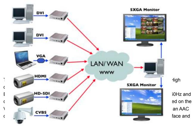
Figure 1: Multiple PC and Video HD encode
