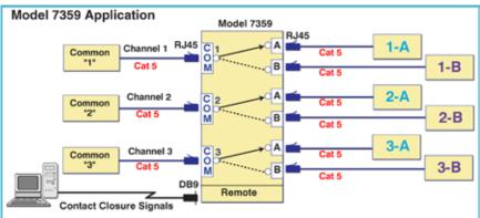
iii. IP Addressable - Remote control of the switch position is from a 10 Base-T/100 Base-TX LAN Ethernet environment. Users communicate with the switch via a TELNET session. The user setup allows assignment of an IP address for the switch unit.
