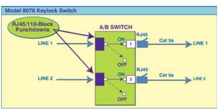
**B)** Lockout – The advantage of the lockout feature is that the user can lockout the switch position remotely and be assured that the switch is operating as prescribed.
