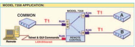
v. Code Operated - The switch position and lockout status can be changed through the data stream on the COMMON port.
