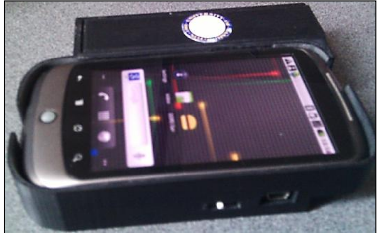
A photograph of the current design. The DDRS features snap-on functionality, USB and Bluetooth connections, as well as a built-in laser. It uses the phone’s on-board GPS sensor for location tracking.
