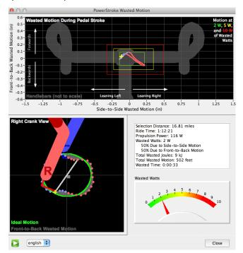
PowerStroke takes advantage of the high-speed data bus design of the iBike Newton line of power meters, and the accelerometer and pressure sensors used exclusively by the iBike Newton line. PowerStroke records data 16 times per second – ten times faster than any power meter in the world. This recording rate is so fast that motion can be determined even as the cyclist turns the bike crank. PowerStroke data is processed on a Mac or PC, with new,
