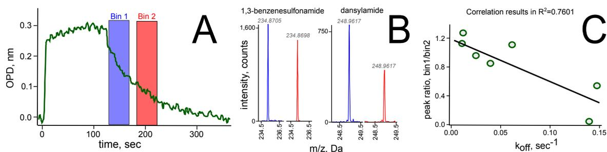
**Figure 3: Results of binned AC-MS** In A the total, label-free NPOI signal is shown for the mixture of sulfonamides interacting with an immobilized CAII surface. The shaded areas shown indicate the ‘bins’ of eluent which were collected. B shows an example mass spectra segments comparing the peaks between 1,3-benzenesulfonamide and dansylamide. While C shows the inverse linear relationship between peak ratio between bin 1 to bin 2 and  $k_{off}$ .
