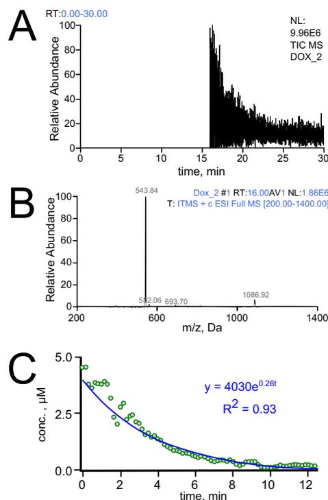
**Figure 2: Real time elution measurement.** A Total ion current spectrum from the eluent is shown starting during the dissociative phase. B Mass spectrum at 16 minutes. C Dox ions quantified over time in XIC mode.
