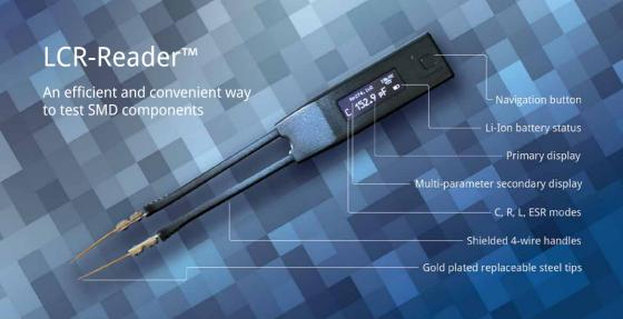
LCR-Reader™ is a professional quality, low cost LCR and ESR-meter. It provides the perfect solution for testing and identifying Surface Mount Devices (SMD), as well as troubleshooting complex electronic systems.
