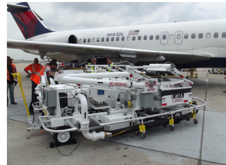
An 800 GPM (3000 lpm) BETA Fluid Systems wide-body hydrant cart is preparing to fuel an aircraft at Atlanta's Hartsfield International Airport in February, 2014.
