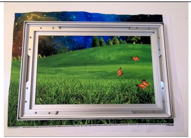
The frame is centered onto the chosen textile. Leave a minimum of 2" bleed all around the frame.
