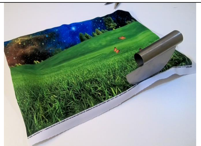
Insertion of the textile in the extrusion channel.
