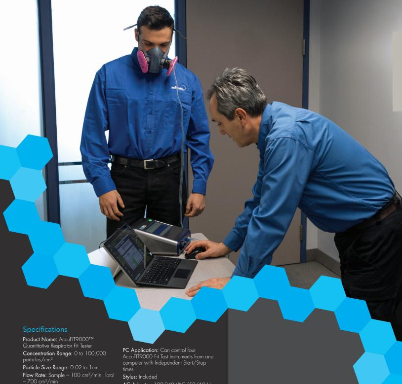
Temperature Range: 15°C to 35°C Fit Factor Measurement: Direct measurement of fit factor (Cout/Cin)Alcohol: Reagent-Grade 2-propanol Display: 7" colour touchscreen Power Supply: AC adapter
