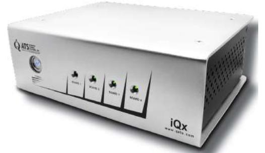
The iQx™ system is equipped with input ports for up to eight air temperature/velocity sensors, four J type thermocouples, two pressure sensors and one humidity sensor. These can be positioned in different locations within a system under test, such as an electronic enclosure.
