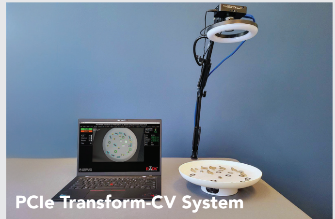
PC-based Systems: Appropriate NVIDIA GPU-based PC, Monitor, High-Res, High-Frame Rate Camera with Interface Module (if needed), Illuminator, Turntable-based Assembly Line Emulator
